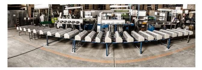
This device is designed in such a way that selects the best performance by having a very strong controller and several sensors and continuous monitoring of the ambient and internal temperature. This device is a combination of an air curtain device and an air purifier. As long as the door is closed, the device starts disinfecting and sterilizing the air by UVC lamp and as soon as the device door is opened, it will change the mode and work in air curtain mode. This device has two working modes:
